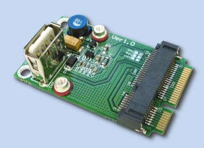
The MM2U half to full mini card is a converter tool for minicard interface.
