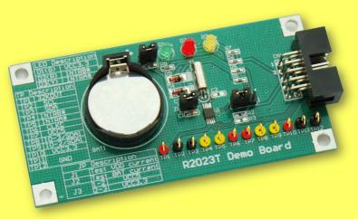
The new R2023T Real Time Clock Demo Board is a compact, easy to control Real Time Clock, ideal for use when setting up a real-time control system or for use when date stamping is required for various monitoring applications.
