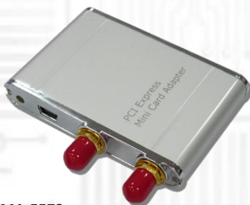
USBMA-5572 (Wireless USB Mini Card Adapter ) x1 with Ralink® RT5572 WiFi Card x1 IPX to RP-SMA cable x2
